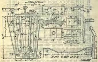
Fig. 28.—Details of Girder Rail Fastenings.
